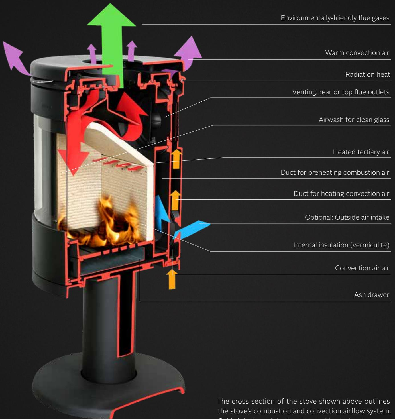
The cross-section of the stove shown above outlines the stove's combustion and convection airflow system. Cold air is drawn into the stove and heated as its passes through the cast iron channels (the heated air washes the glass keeping it clean, clear and free from soot). The hot air also provides perfectly heated combustion air (in addition the heated tertiary air aids secondary combustion of any smoke and gasses, increasing efficiency and reducing the environmental impact).
