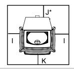
Use a noncombustible floor protector extending beneath appliance and to the front/sides/rear as indicated. Measure front distance (K) from surface of glass door. Approved for use with Type 1 hearth pad.
