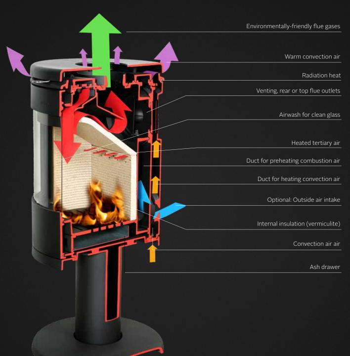
The cross-section of the stove shown above outlines the stove's combustion and convection airflow system. Cold air is drawn into the stove and heated as its passes through the cast iron channels (the heated air washes the glass keeping it clean, clear and free from soot). The hot air also provides perfectly heated combustion air (in addition the heated tertiary air aids secondary combustion of any smoke and gasses, increasing efficiency and reducing the environmental impact).
