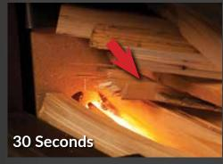
Hot surface igniter blows 1,400 degree heated air into the firebox, igniting the wood.
